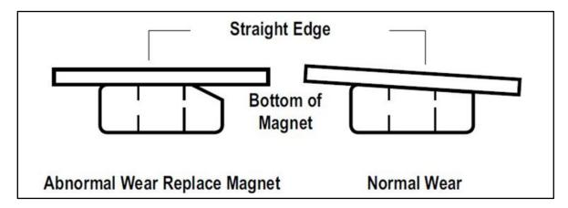
Even if wear is normal as indicated by your straightedge, the magnets should be replaced if any part of the magnet coil has become visible through the friction material facing of the magnet. It is also recommended that the drum armature surface be refaced when replacing magnets.
