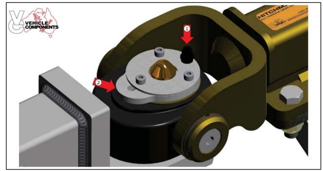
Push down the button 1 and push the locking mechanism back 2. When the locking mechanism is all the way back, release the button while holding the mechanism to ensure it does not spring back to the locked position.
