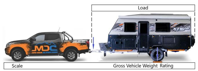
**GCWR (Gross Combination Weight) Rating:** The total permissible mass that can be supported by the wheels/ tires of the Tow Vehicle and Trailer Combination. This includes whatever you add as payload (e.g. water, gas, equipment, and luggage), and total weight of the tow vehicle. The GCW Rating must not be exceeded.
