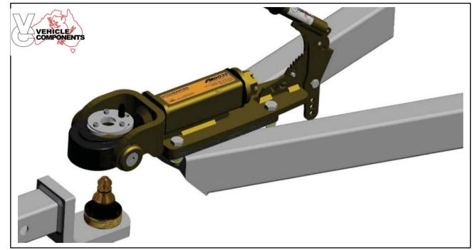
Lift the coupling up off the tow pin.
