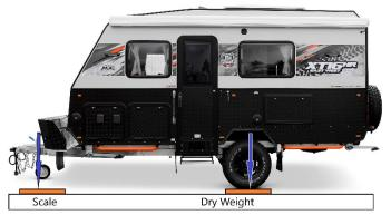
**GVW (Gross Vehicle Weight) Rating:** The total permissible mass of the Trailer. This includes the coupling mass and whatever you add as payload (e.g. water, gas, luggage) up to the specified rating. The GVW Rating must not be exceeded.
