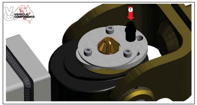
Make sure the tow pin is seated inside the universal and the tow pin top is sticking out of the locking mechanism (see below). Press the button (1) to release the locking mechanism there will be an audible locking noise at which point the mechanism will return to the initial position as shown in step 1. Verify the pin is correctly through the mechanism and assemble the cap. If the cap will not fit, check the locking mechanism is in the correct locked orientation.
