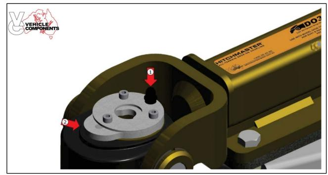
Push down the button (1) and push the locking mechanism back (2). When the locking mechanism (2) is all the way back, release the button (1) locking the plate in place
