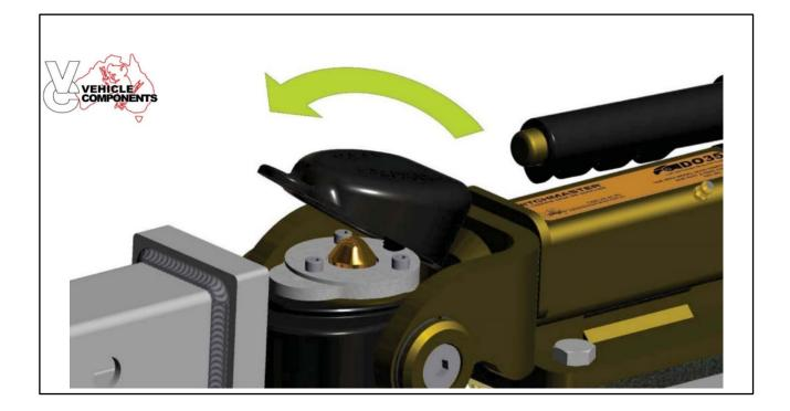
Make sure the dust cap is securely connected to the bump cover. This is done by locating the rear lip on the dust cap onto the groove of the bump cover and then pushing it in a downward motion until the dust cover is secure (there should be a slight click when it has been assembled correctly) Test if the dust cover is connected to the bump cover by applying a slight upward force to the dust cover, it shouldn't separate. This procedure should be applied if you are uncoupling or coupling up.
