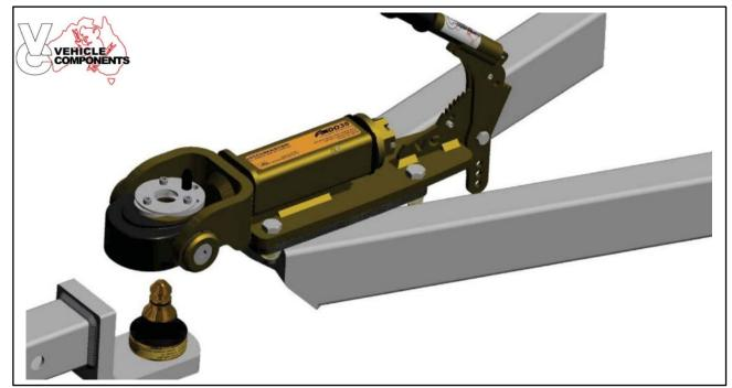
Offer up the tow pin to the coupling making sure the tow pin cover is removed and there is no visible debris on it. Locking plate should be in unlocked position as shown. Lower the coupling onto the tow pin.
