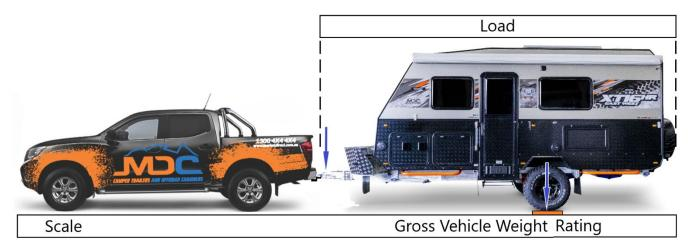
GCWR (Gross Combination Weight) Rating: The total permissible mass that can be supported by the wheels/ tires of the Tow Vehicle and Trailer Combination. This includes whatever you add as payload (e.g. water, gas, equipment, and luggage), and total weight of the tow vehicle. The GCW Rating must not be exceeded.
