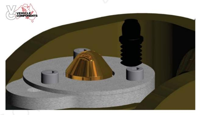
Detail view of pin through locking mechanism.
