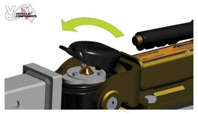
Make sure the dust cap is securely connected to the bump cover. This is done by locating the rear lip on the dust cap onto the groove of the bump cover and then pushing it in a downward motion until the dust cover is secure (there should be a slight click when it has been assembled correctly) Test if the dust cover is connected to the bump cover by applying a slight upward force to the dust cover, it shouldn't separate.
