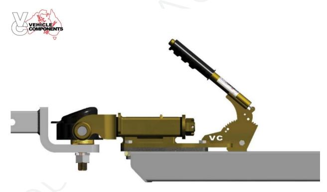
Make sure the handbrake is applied prior to coupling and uncoupling.
