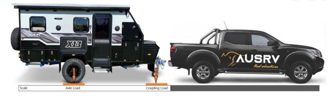
**GVW (Gross Vehicle Weight) Rating:** The total permissible mass of the Trailer. This includes the tongue/coupling mass and whatever you add as payload (e.g. water, gas, luggage) up to the specified rating. The GVW Rating must not be exceeded.
