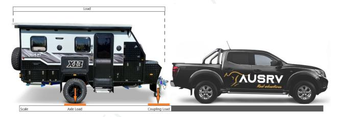
**GCWR (Gross Combination Weight) Rating:** The total permissible mass that can be supported by the wheels/ tires of the Tow Vehicle and Trailer Combination. This includes whatever you add as payload (e.g. water, gas, equipment, and luggage), and total weight of the tow vehicle. The GTM Rating must not be exceeded.
