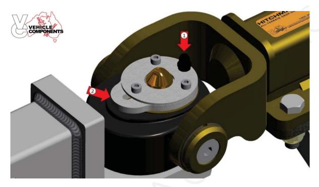
Push down the button 1 and push the locking mechanism back 2. When the locking mechanism is all the way back release the button while holding the mechanism to ensure it does not spring back to the locked position.
