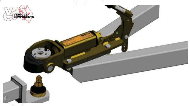
Lift the coupling up off the tow pin.
