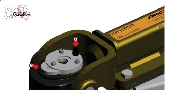
Push down the button (1) and push the locking mechanism back (2). When the locking mechanism (2) is all the way back, release the button (1) locking the plate in place
