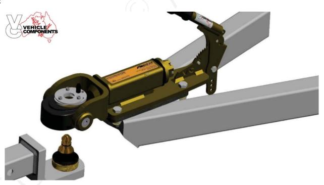
Offer up the tow pin to the coupling making sure the tow pin cover is removed and there is no visible debris on it. Locking plate should be in unlocked position as shown. Lower the coupling onto the tow pin.
