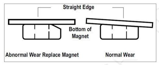
Even if wear is normal as indicated by your straightedge, the magnets should be replaced if any part of the magnet coil has become visible through the friction material facing of the magnet. It is also recommended that the drum armature surface be refaced when replacing magnets.
