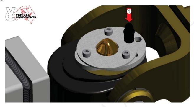
Make sure the tow pin is seated inside the universal and the tow pin top is sticking out of the locking mechanism (see below). Press the button (1) to release the locking mechanism there will be an audible locking noise at which point the mechanism will return to the initial position as shown in step 1. Verify the pin is correctly through the mechanism and assemble the cap. If the cap will not fit check the locking mechanism is in the correct locked orientation.
